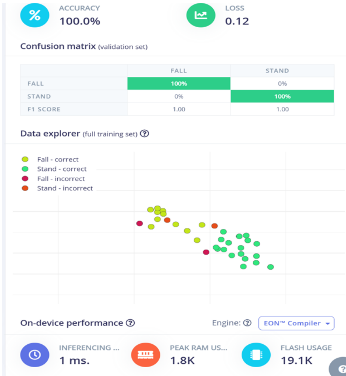
Figure 8: Training performance showing 100% validation accuracy with 0.12 loss. On-device metrics: 1ms inferencing time, 1.8K peak RAM usage, and 19.1K flash usage
